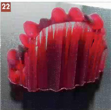
This was printed in Freeprint Cast material
